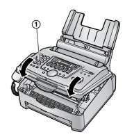
8 Pull the tension plate forward (①), then reinsert the recording paper (②). • Before re-inserting, make sure to fan and straighten the recording paper.
